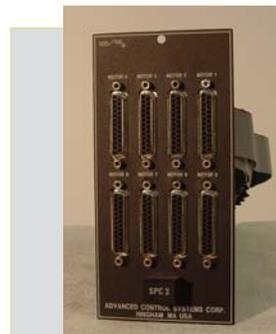
The *Step-Pak* **SPC-3 Interface Module** provides eight front panel connectors for connection to an external indexer/controller. The SPC-3 also provides differential receivers on step and direction inputs for all eight channels.
