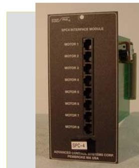
The *Step-Pak* **SPC-4 Interface Module** provides eight RJ-45 front panel connectors for the connection of an external eight channel indexer or controller. The SPC-4 facilitates system wiring through the use of standard cables
